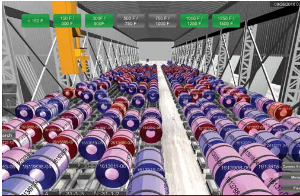
A coil tracking application uses the position of the crane given by the positioning sensors to keep track of coils, even as they cool, eliminating the requirement for pen-and-paper tracking.
