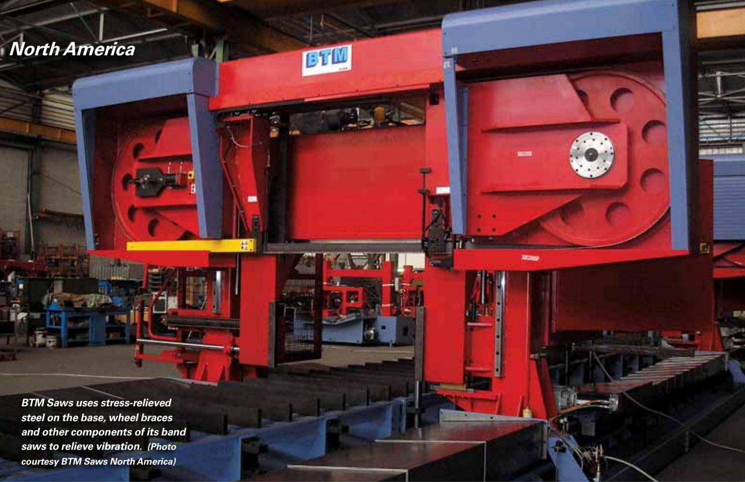
BTM Saws uses stress-relieved steel on the base, wheel braces and other components of its band saws to relieve vibration. (Photo courtesy BTM Saws North America)
