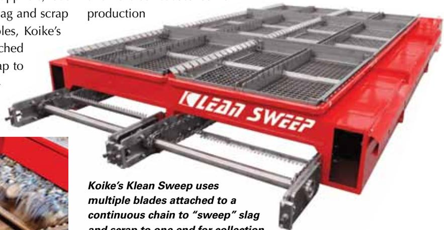
**Koike's Klean Sweep uses multiple blades attached to a continuous chain to "sweep" slag and scrap to one end for collection into in-floor hoppers or portable bins. (Photo courtesy Koike)**
