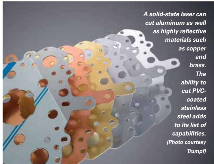
*A solid-state laser can cut aluminum as well as highly reflective materials such as copper and brass. The ability to cut PVC-coated stainless steel adds to its list of capabilities. (Photo courtesy Trumpf)*
